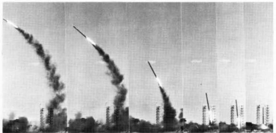
A stuck valve in one of the four clustered engines caused the third rocket launched to arc over for a spectacular crash in the Luvua river valley.
